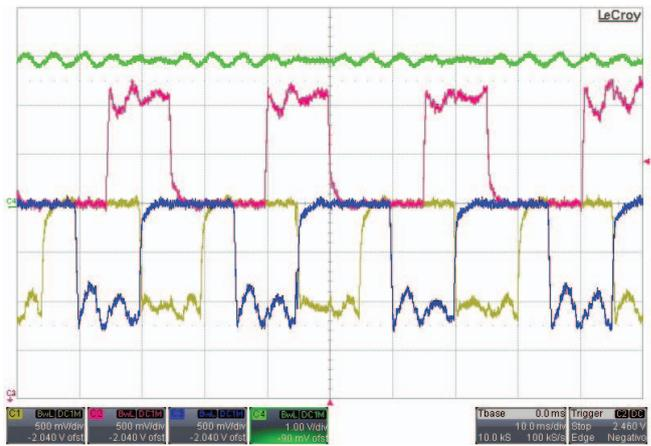
Figure 6 Healthy mode operation @ 300 rpm, 8 Nm: Phase-A, Phase-B, and Phase-C measured currents (yellow, red, blue); motor speed (green); current is scaled to 15A/div.
