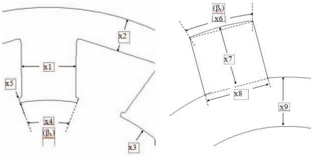
Figure 2 Design variables of the Switched Reluctance motor: Stator (left) and rotor (right) details.
