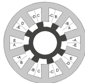
Figure 1 Cross-section and winding distribution of the five-phase 10/8 SR motor.
