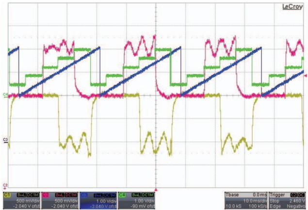
Figure 5 Healthy mode operation @ 300 rpm, 8 Nm: Phase-A and Phase-B measured currents (yellow, red), commutation sector (green), electrical position (blue); current is scaled to 15A/div.
