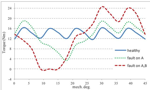
Figure 3 Optimized design: torque vs. rotor position in the healthy and faulty mode operation (FE analysis).
